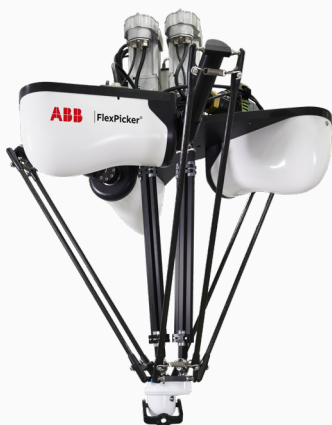
— IRB 365 FlexPicker® five axis Delta robot fastest for lightweight product picking
