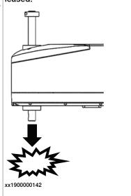
3 Release the holding brake of all axes by pressing the brake release button.
