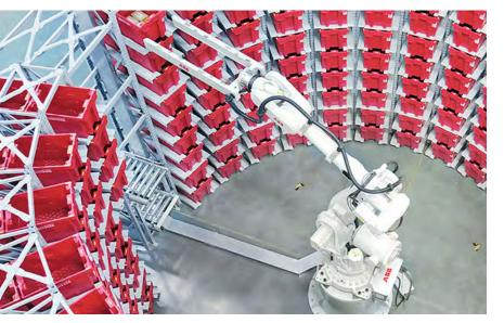
The FlexBuffer™ is a modular cell, that offers additional functionality to the traditional automated storage and retrieval systems.
