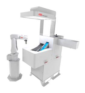
FlexLoader FP 100 is a compact and proven function package for machine tending and assembly operations, pre-configured and ready to use for fast integration. The solution is a combination of robust hardware and intelligent vision software. It is an ideal solution to tend small workpieces to transfer machines with short cycle times.
